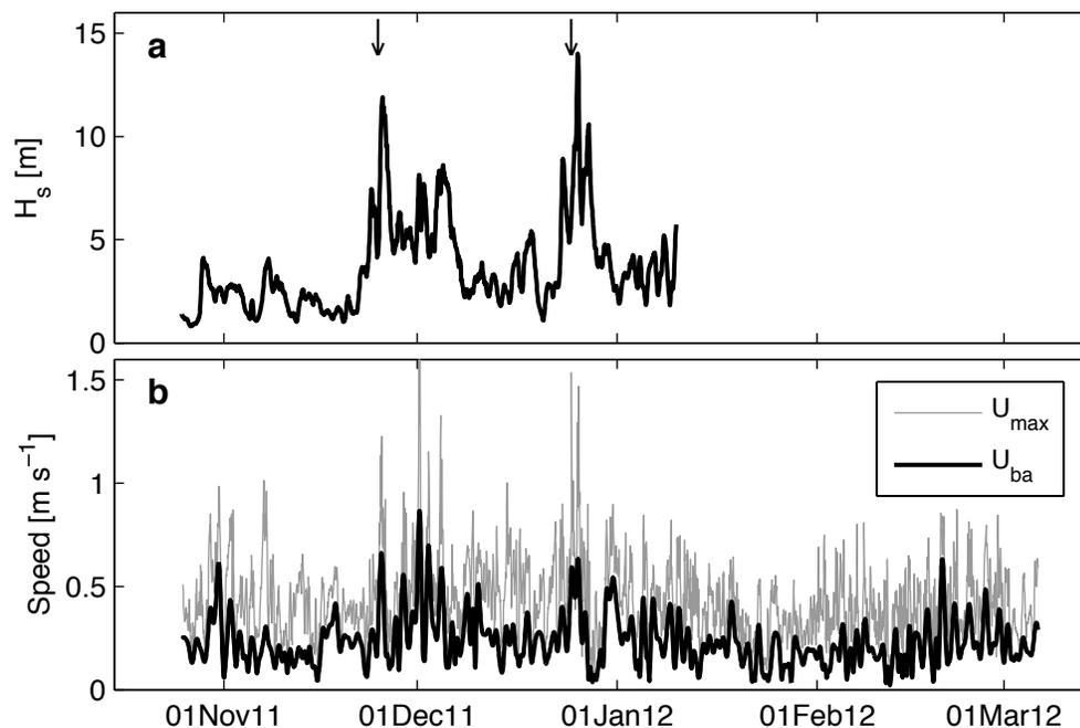
**Figure 2.** Havsul I offshore wind farm. Position 62°50'07"N 06°08'14"E. Time series of a) significant wave height, b) magnitude of the maximum hourly velocity ( $U_{max}$ , gray) and the depth-averaged 25-hour low-passed velocity ( $U_{ba}$ , black) at Havsul-I region measured at approximately the 130 m isobath. The arrows in a) mark the storms Berit and Dagmar in late November and December 2011, respectively.
