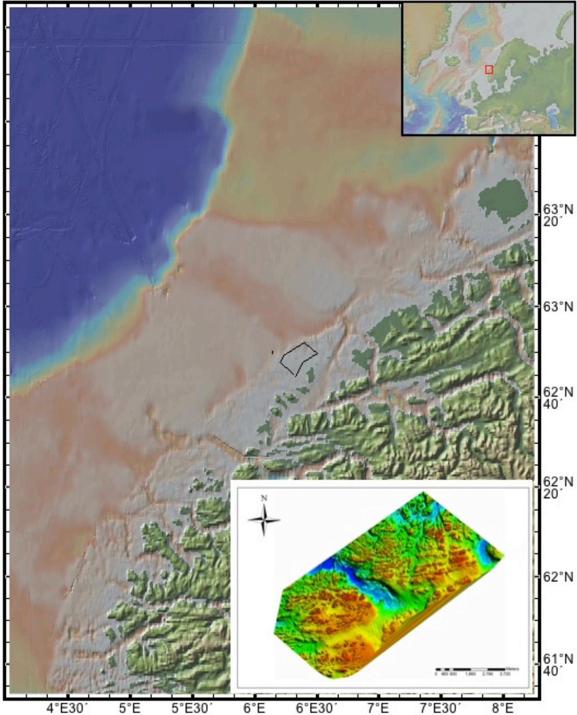
**Figure 1.** Havsul I offshore wind farm. The site is indicated with a black rectangle. The insert at the lower right is a multibeam bathymetric map of the actual area.
